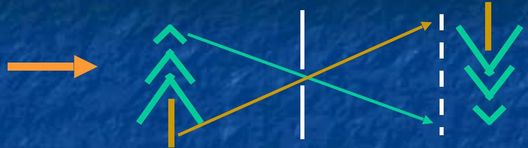
Critical advantage of pinhole camera is that you do not need a lens
